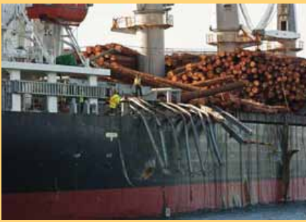
Broken cargo stanchions on the log carrier Dry Beam , February 2012. The vessel issued a mayday after 11 m seas and hurricane-force winds damaged and endangered the ship northwest of Vancouver Island. Enbridge’s associated oil tankers would sail through these same seas. PHOTO: D. STONE.
