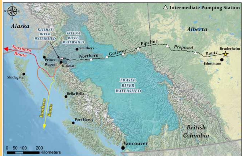
Figure 2.2 The proposed pipelines would run 1,172 km (727 miles) through a 1-km wide clearcut corridor from Bruderheim, Alberta to Kitimat on BC's north coast. The pipelines will be buried along most of the route, except at certain river crossings, and at the Clore and Hault tunnels.
